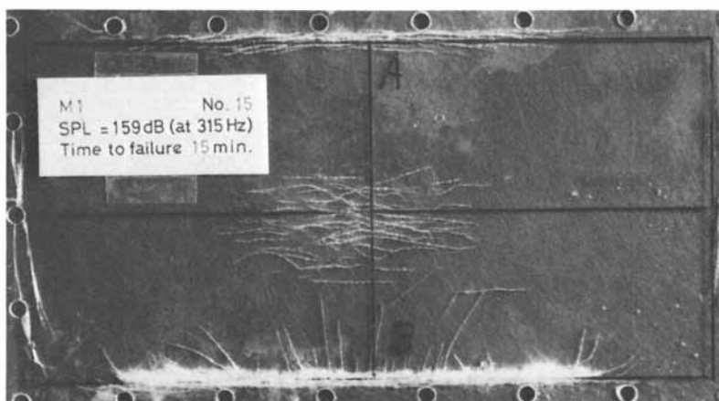
Figure 4. Failure pattern for test panel with a glass-fiber mat layer
