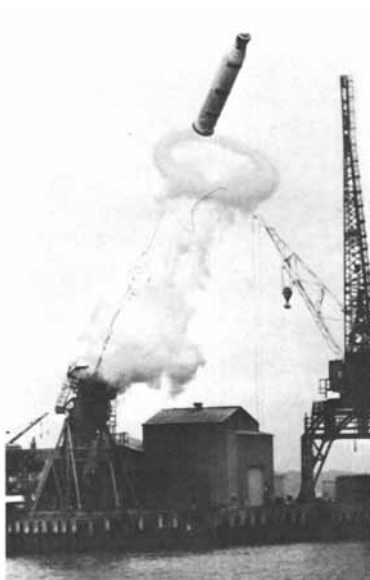
Figure 18. "Cold Launch" seal test using compressed gas for propellant
