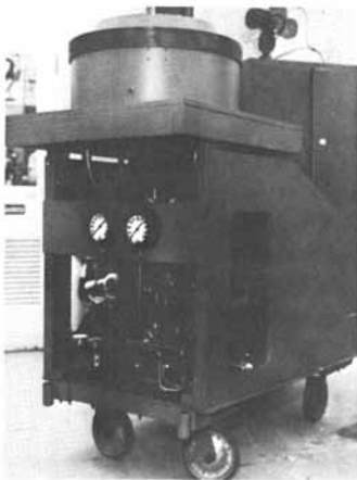
Figure 12. Two-foot-diameter launch seal test apparatus
